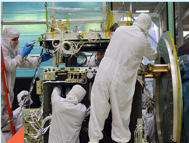
NASA engineers conduct a fit test on the ATLAS instrument of the ICESat-2 mission
